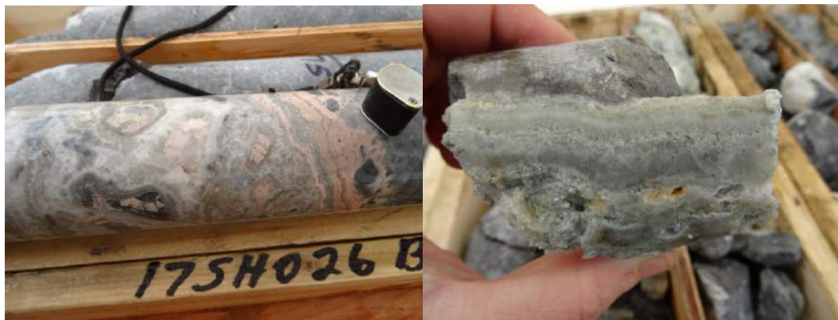
2017 Drill Core Photos: The Rhodo Breccia (17SH026; left) and the Greenbaum Vein/Breccia (17SH027, right). Both exhibit gangue-mineralogy and epithermal textures related to high-grade gold mineralization observed elsewhere along the Shumagin Gold Zone.
